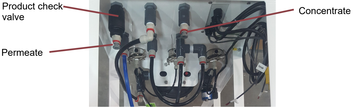
System rear view
